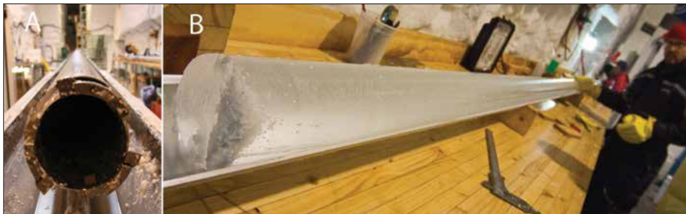
Figure 1: Drilling an ice core. A) The drill head of the NEEM drill (photo: J.P. Steffensen). B) A freshly drilled 3.5-m ice core section at NEEM (photo: T. Burton).
